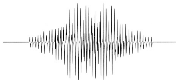
Figure 3. Computer-simulated EPR spectrum with the following splittings (line width of 0.1 G, and modulation of 0.1 G): 11.73 (1:3:3:1), 5.10 (1:1:1), 3.71 (1:1), 2.58 (1:1:1), 1.26 G (1:1).
